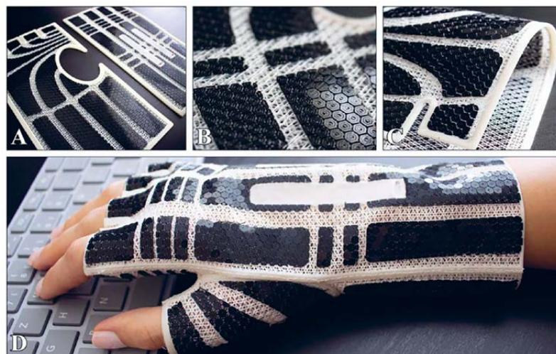
Figure 4: 3D printed glove: A) sewing pattern printed from two materials, B) surface design of the glove, C) flexible sewing pattern with inner lining, D) pattern parts sewn together to form a three-dimensional garment [4]
