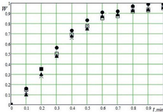
Figure 10: Experimental data of moisture content in medical cotton wool
