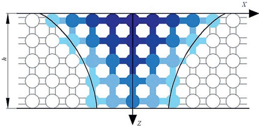
Figure 2: Discrete model of fluid passage through material
