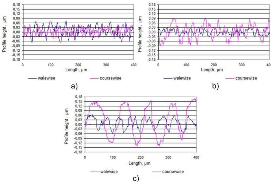
Figure 3: Roughness profiles of wool knitted fabric samples: a) single plain; b) 1x1 rib 380 g/m<sup>2</sup>; c) 1x1 rib 450 g/m<sup>2</sup>
