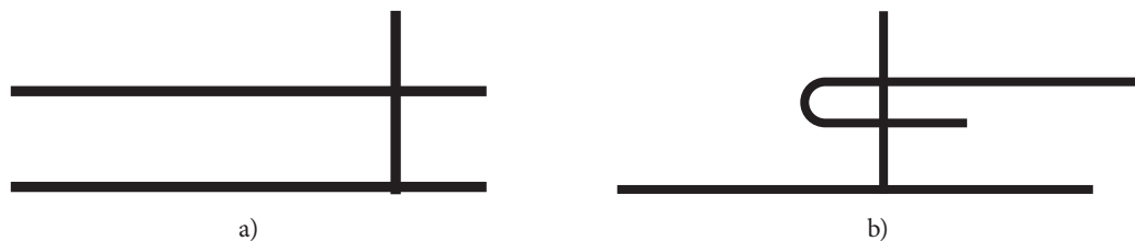
Figure 2: Seam configuration: a) superimposed seam (SSa) and b) lapped seam (LSd)
