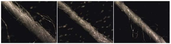
ring spun yarn rotor spun yarn air-jet spun yarn *Figure 2: Tencel™ ring, rotor and air-jet spun yarn images taken with Dino-Lite digital microscope (60× magnification)*
