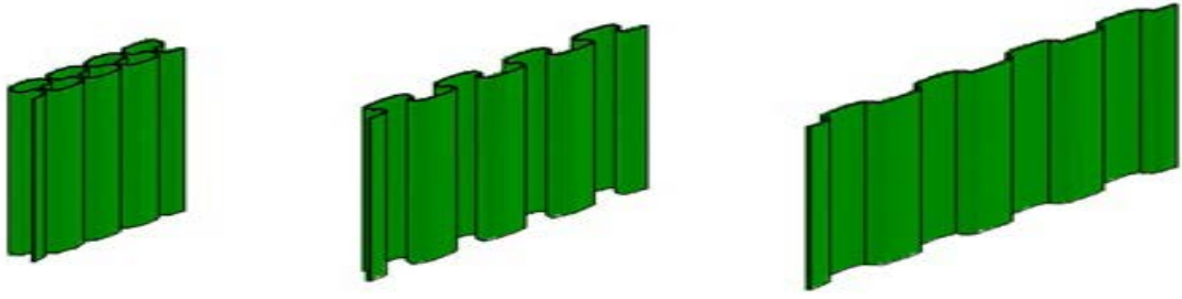
Figure 7: Three states of tension of rib stitch structure sample represented in macro-models
