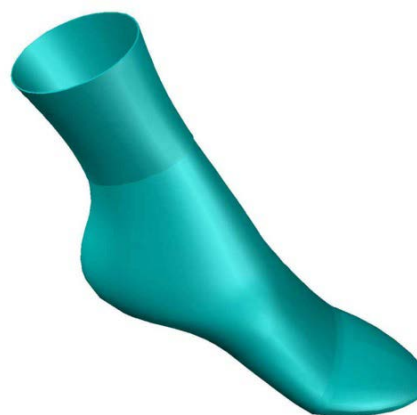
Figure 1: 3D model of sock represented as shell with homogenised properties within system of three-dimensional modelling
