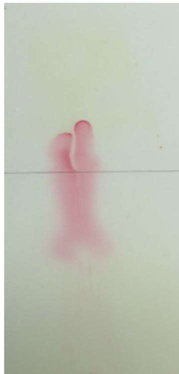
Figure 10: TLC plate for the synthesised dye after the solvent almost reached the top of the plate
