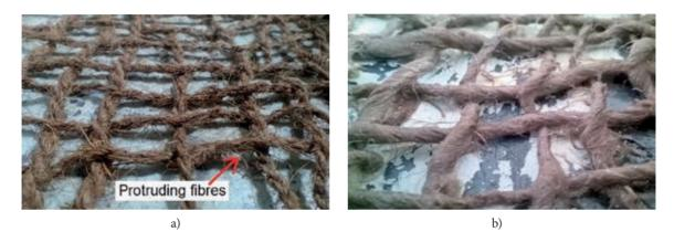
Figure 5: Geomeshes under zero-infiltration conditions: a) coir geomeshes b) Jute geomeshes
