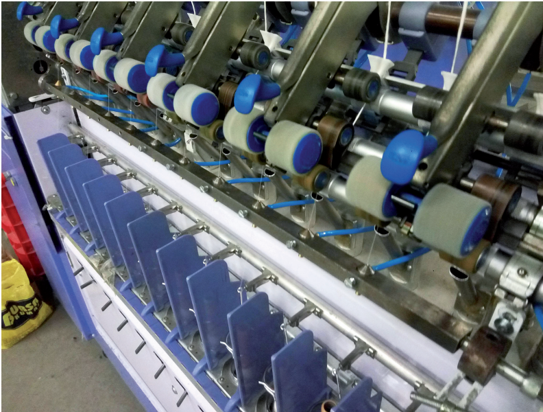
Figure 4: Jet-ring air nozzles mounted on a conventional ring spinning machine
