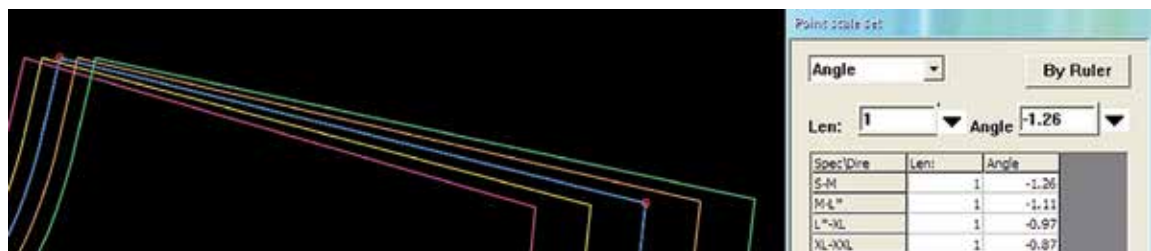
Figure 6: Shoulder grading of T-shirt spec A by actual angle grading in Boke CAD
