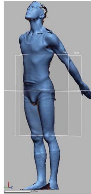
Figure 4: Multiple scan's meshes fused together
