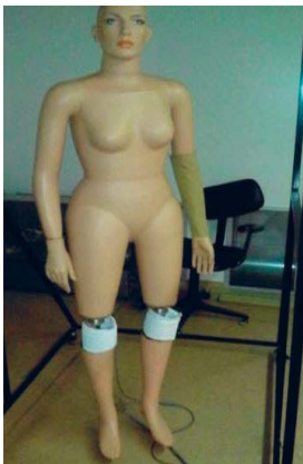
Figure 2: Thermal manikin Maria with left forearm covered with sample of firefighter protective clothing
