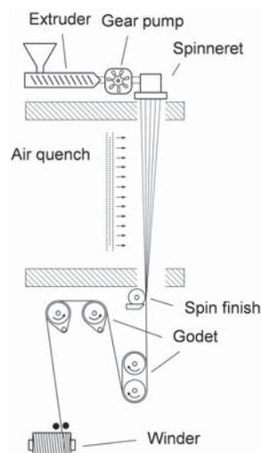
Figure 1: Lab scale melt spinning plant
