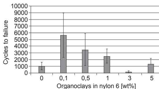
Figure 3: Abrasion resistance with bechlenberg
