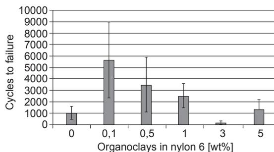
Figure 3: Abrasion resistance with bechlenberg
