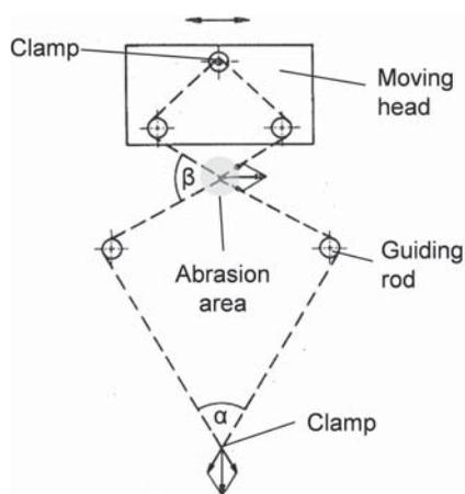
Figure 2: Bechlenberg test device
