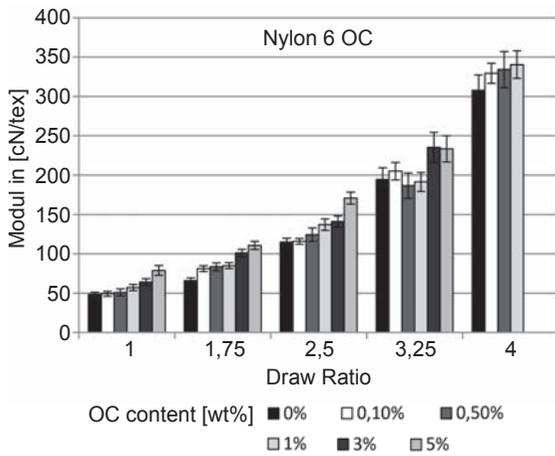
Figure 5: Module over draw ratio ( $\lambda_D$ ) and organo-clay (OC) content
