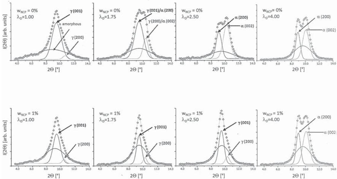
Figure 6: Crystal structure over draw ratio ( $\lambda_D$ ) and organoclay (OC) content
