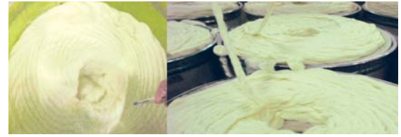
Figure 3: Flattened bottom sliver coils at speedframe creel
