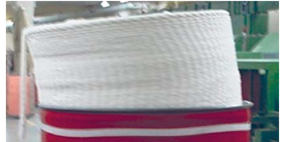
Figure 4: Can-spring buckling on sliver storage in older can
