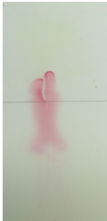
Figure 10: TLC plate for the synthesised dye after the solvent almost reached the top of the plate
