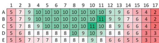
Figure 3: Illumination in W/m 2 , measured in middle of each sample position
