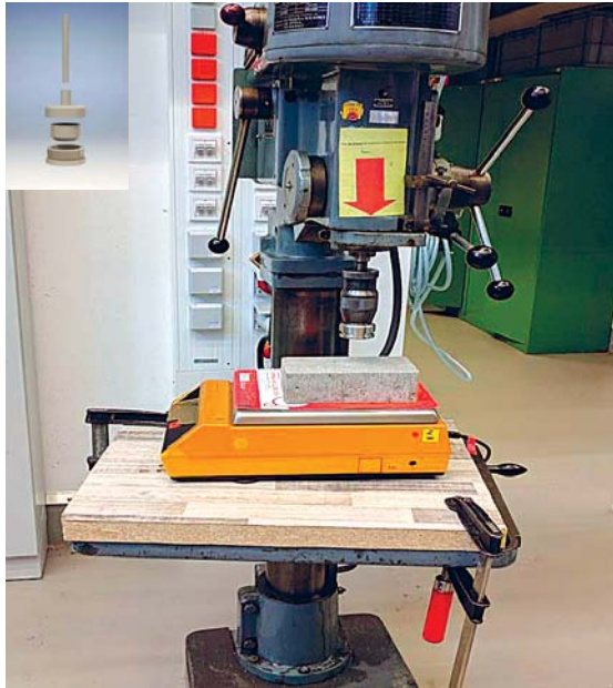
Figure 1: Pillar drilling machine used for tests reported here (left panel) and sketch of sample holder taken from Martindale abrasion tester (right panel)
