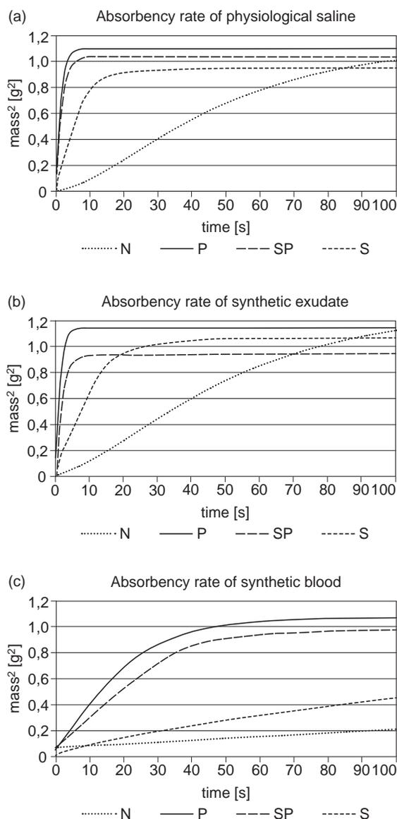
Figure 1: The square mass data of physiological saline (a), synthetic exudate (b), and blood solution (c) rise on non-treated (N), oxygen plasma (P), sol – gel /Ag (S), and sol – gel/Ag and plasma (SP) treated samples
