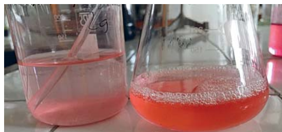
Slika 10: Odpadna voda, onesnažena s tiskarsko barvo po čiščenju z Al_2O_3 , in izhodiščna odpadna voda pred čiščenjem Figure 10: Printing ink wastewater after treatment with Al_2O_3 and initial wastewater before treatment
