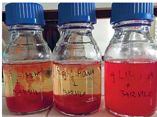
Slika 1: Odpadne vode, onesnažene z barvilom po čiščenju z 10, 7,5 in 5 g/l limoninih olupkov Figure 1: Wastewaters polluted with dye after treatment with 10, 7.5 and 5 g/l lemon peels
