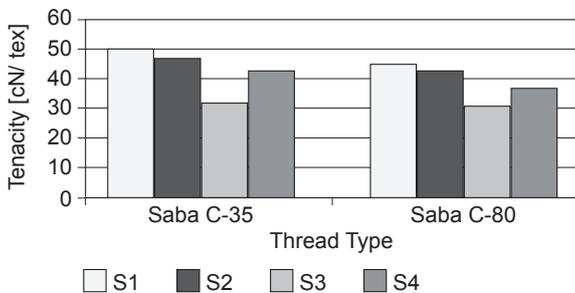
Figure 9: Tenacity of thread at 4000 rpm of machine
