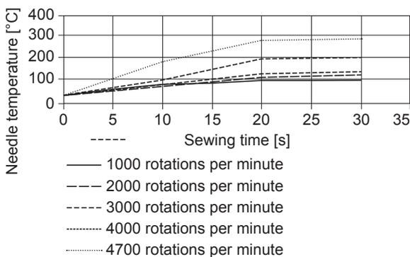
Figure 4: Needle temperature (with thread Saba C-80)
