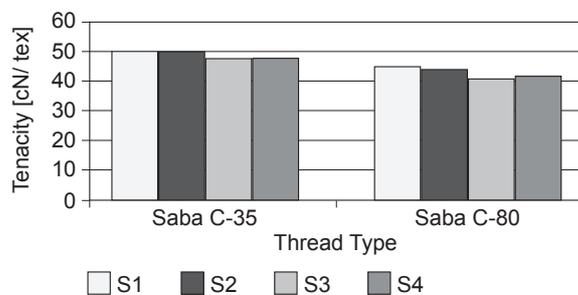
Figure 7: Tenacity of thread at 2000 rpm of machine
