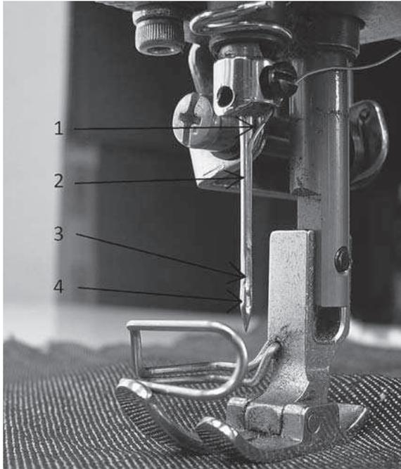
Figure 1: Sewing needle with inserted thermocouple
