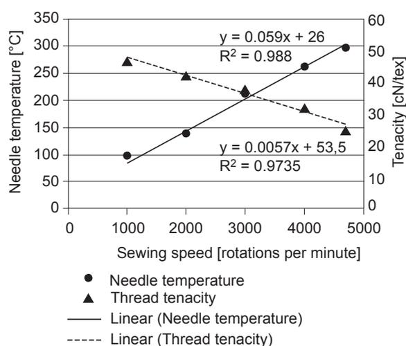
Figure 13: Needle temperature and tenacity of sewing thread
