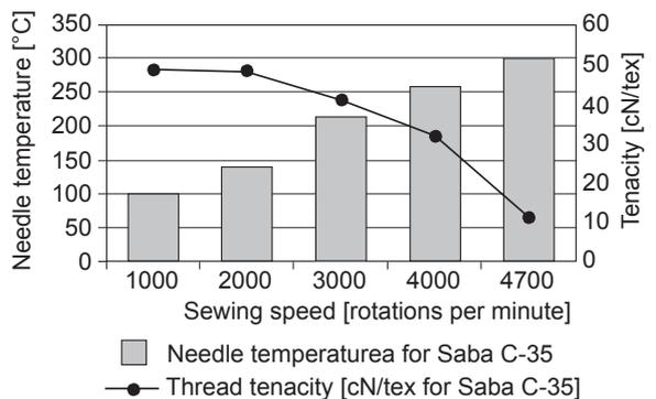
Figure 11: Needle temperatures and tenacity of thread at section S3 for thread Saba C-35
