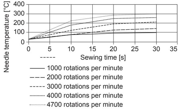
Figure 5: Needle temperature with thread Saba C-35
