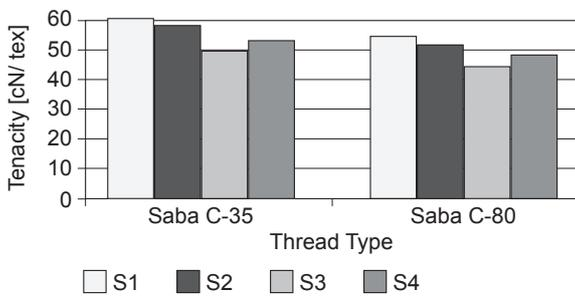
Figure 8: Tenacity of thread at 3000 rpm of machine
