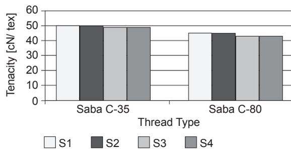
Figure 6: Tenacity of thread at 1000 rpm of machine
