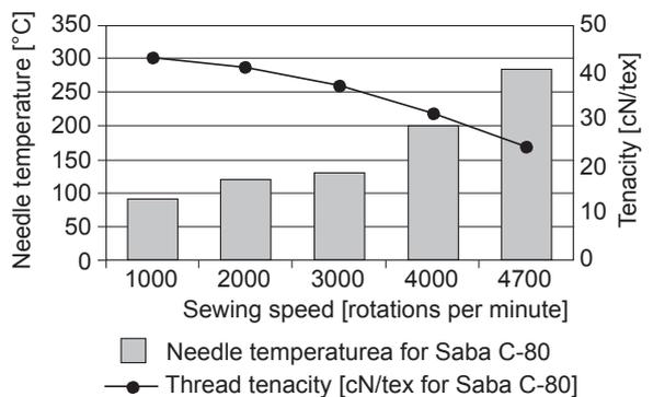
Figure 12: Needle temperatures and tenacity of thread at section S3 for thread Saba C-80
