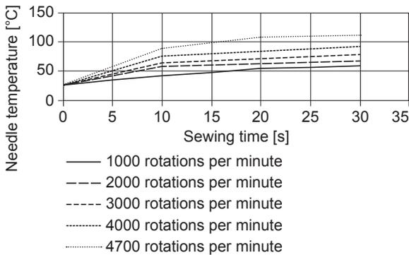
Figure 3: Needle (without thread) temperature
