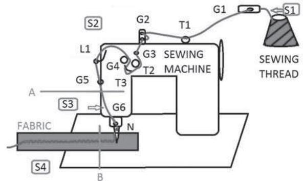
Figure 2: Passage of sewing thread through sewing machine
