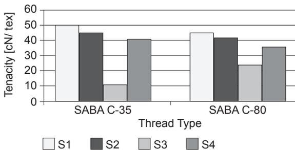
Figure 10: Tenacity of thread at 4700 rpm of machine
