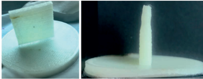
Figure 7: Examples of broken 3D-printed object (left) and deformed 3D-printed object (right) after mechanical testing
