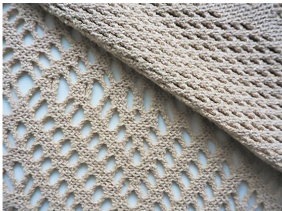
Slika 12: Snutkovno pletivo Karl Mayer s kvačkanim videzom (vir: https://www.karlmayer.com/en/products/warp-knitting-machines/raschel-machines/rascheltronic%C2%AE/rsjfs-4/1-el/crochet-knit/ )
