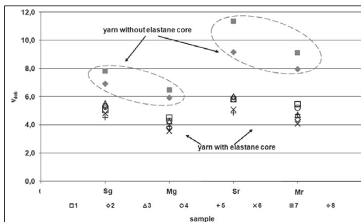
Figure 3: Fabric thickness interlacing factor,  $v_{deb}$ , of dense and loose, dry, and dry and wet relaxed (consolidated) structures made from yarns without elastane core and yarns with elastane core
