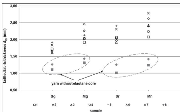
Figure 1: Comparison of fabric thickness,  $d_{pl0}$ , of dense and loose, dry, and dry and wet relaxed (consolidated) structures
