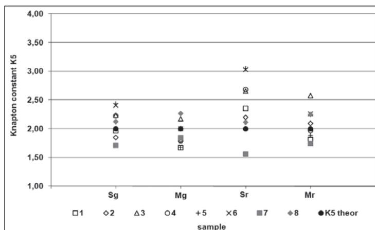
Figure 2: Comparison of Knapton constant,  $K_5$ , of dense and loose, dry, and dry and wet relaxed (consolidated) structures
