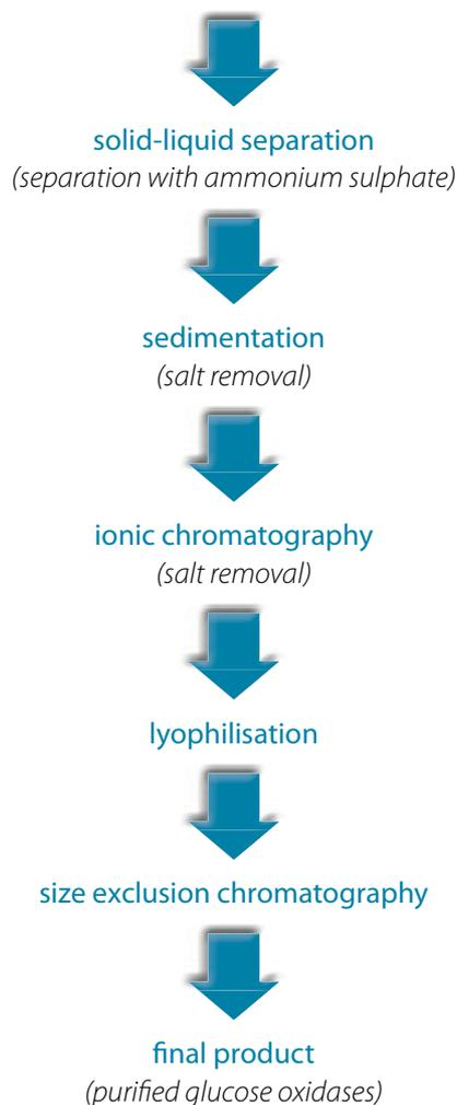
Figure 3: General set of processes to produce pure glucose oxidases [5]
