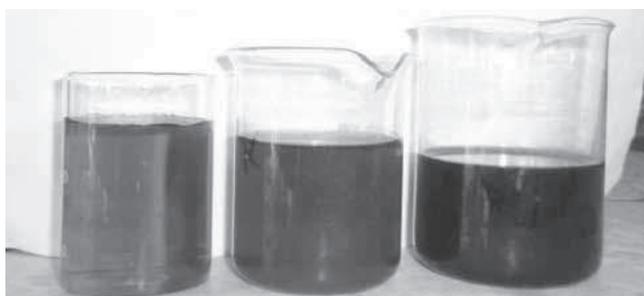
Figure 2: Sample of permeate (purified water within MBR system), sample from bio-unit (wastewater after biological treatment) and fed solution
