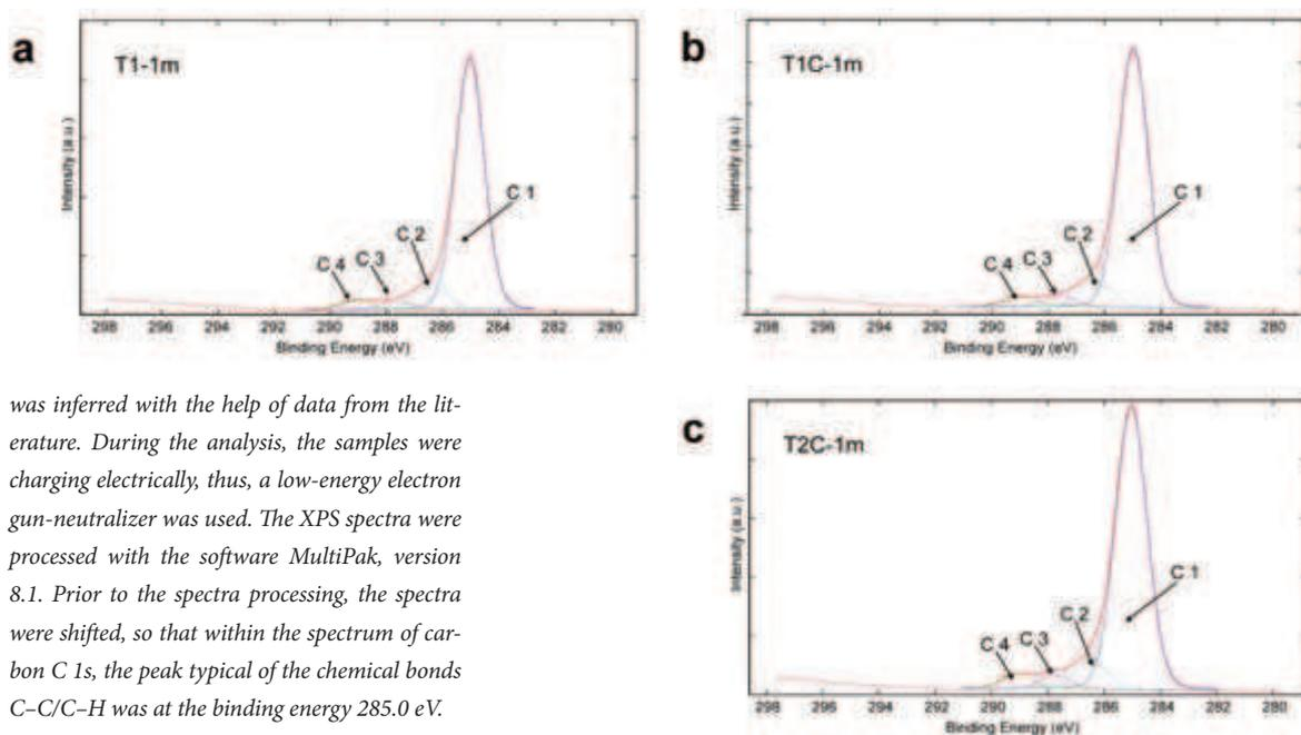
was inferred with the help of data from the literature. During the analysis, the samples were charging electrically, thus, a low-energy electron gun-neutralizer was used. The XPS spectra were processed with the software MultiPak, version 8.1. Prior to the spectra processing, the spectra were shifted, so that within the spectrum of carbon C 1s, the peak typical of the chemical bonds C-C/C-H was at the binding energy 285.0 eV.
