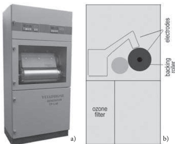
Figure 1: a) laboratory corona plasma apparatus, b) apparatus scheme
