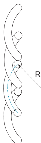
Figure 3: Peirce's loop model (1) – curvature of loop legs
