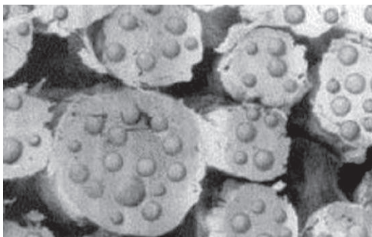
Figure 7: Incorporation of microcapsules into fibres (Outlast®) [15]
