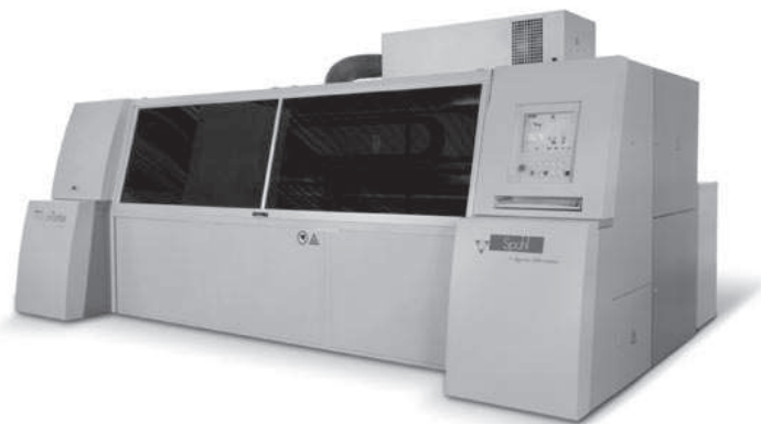
Figure 2.5: The Virtu™ Printer®, a high efficiency ink-jet printing system with continuous UV fixation [28].
